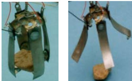
**FIGURE 1:** 4-finger EAP gripper lifting a rock.
