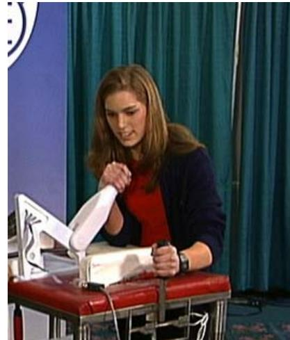
2. The Swiss arm (Figure 4) was able to resist for 4-seconds before losing. This arm was driven by the dielectric elastomer EAP type using multi-layered scrolled actuators that were organized in 4 groups. A photo of one of the group lifting two 5-gallon water containers (about 20-kg) is shown in Figure 5. These actuators were operated similar to
