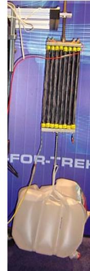
**FIGURE 5:** One of the groups of EMPA's EAP actuators is shown lifting two 5-gallon water containers.
